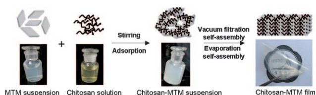
Scheme 1. Fabrication of the artificial nacre-like chitosan-MTM bionanocomposite film. Milky white colloidal chitosan-MTM hybrid building blocks were first prepared by mixing an aqueous suspension of exfoliated MTM nanosheet and an aqueous solution of chitosan and stirring to guarantee full adsorption of chitosan on MTM nanosheets. The chitosan-MTM hybrid building blocks were then aligned into the nacre-like structured composite by self-assembly induced by vacuum filtration or water evaporation.
